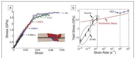
**Figure 2.** (a) Brittle-to-ductile transition as a function of strain rate in silver nanowires. Inset shows snapshot from molecular dynamics (MD) simulation at a strain rate of 10<sup>6</sup>/s.<sup>12</sup> (b) Comparison of measured yield stress and molecular dynamics predictions via nucleation theory.
